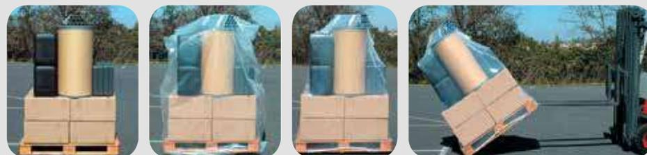
The film takes on the shape of the product by shrinking under the heat produced by the RIPACK® SERIES 3000. The film forms an excellent protective layer and thermal barrier. The objects are held together and the heat transferred is minimal.
